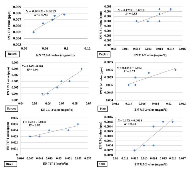
Fig. 4. Correlations between the formaldehyde values measured by EN 717-1 and EN 717-2 methods for different wood species.
