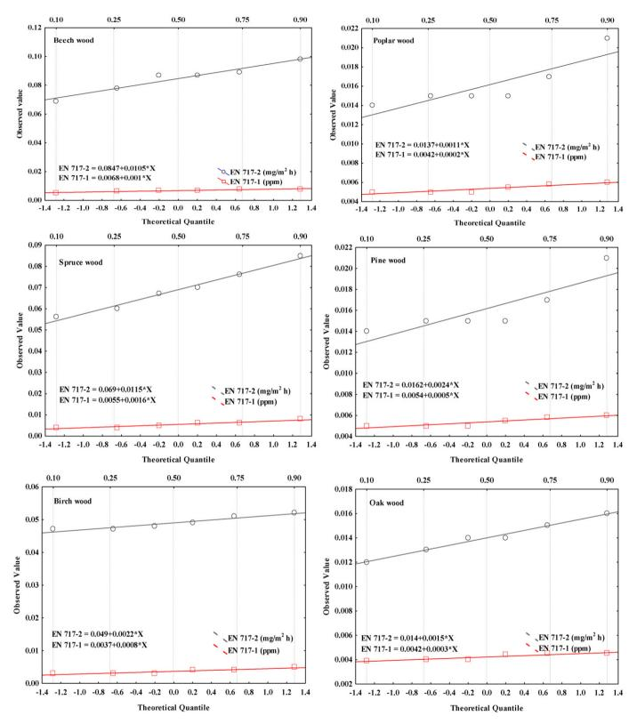
Fig. 3. Normal Q-Q plot distribution of formaldehyde emission from different types of solid wood measured by EN 717-1 and EN 717-2.
