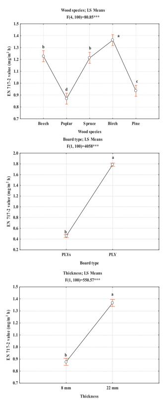
**Fig. 6.** Effect of individual parameters from the manufactured plywood panels on the formaldehyde emission measured by EN 717-2. Vertical bars denote 0.95 CI. Means with the same letter are not significantly different at 0.05 level of probability according to LSD<sub>0.05</sub> test.
