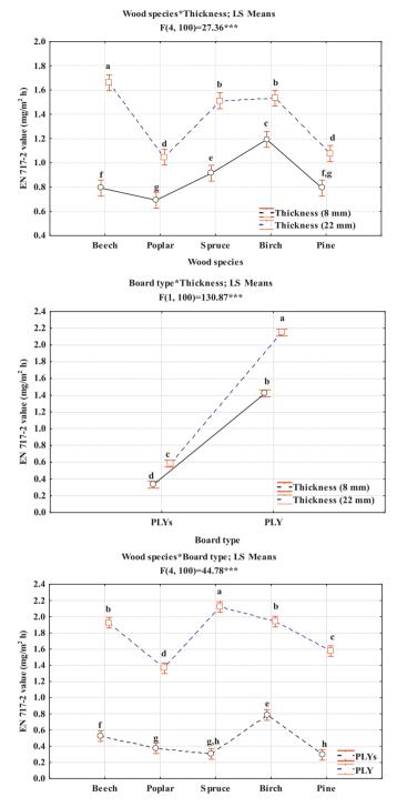
**Fig. 7.** Effect of the interaction between each two parameters from the manufactured plywood panels on the formaldehyde emission measured by EN 717-2. Vertical bars denote 0.95 CI. Means with the same letter are not significantly different at 0.05 level of probability according to LSD<sub>0.05</sub> test.
