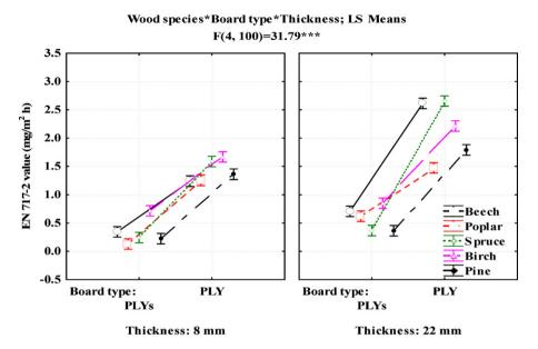
Fig. 5. Effective hypothesis decomposition of the interaction among wood species, board type and thickness and their effects on the formaldehyde emission measured by EN 717-2 method. Vertical bars denote 0.95 CI.
